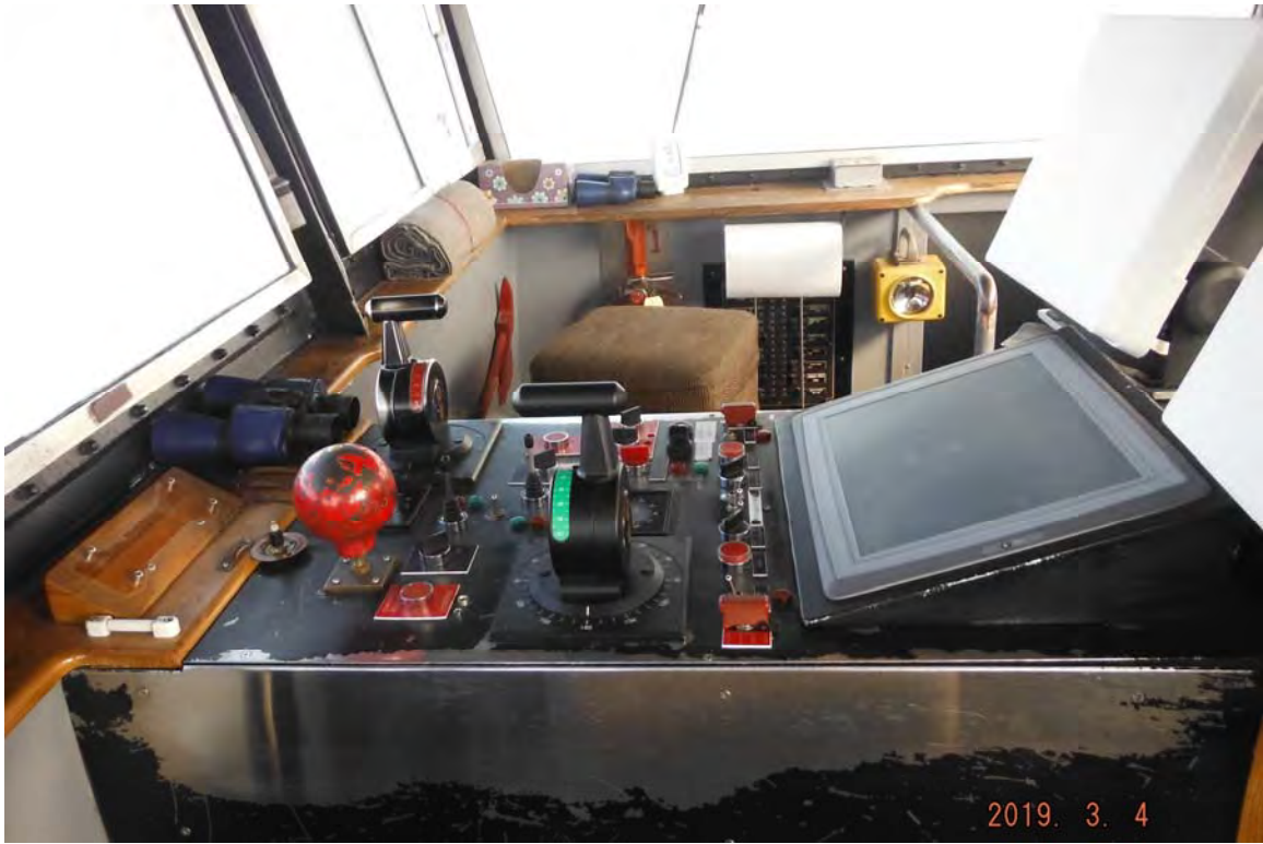
Photo No. 13 Pilothouse Control Console
