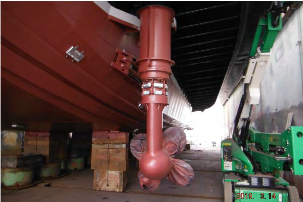
Photo No. 2 No. 1 end Z-drive Unit
